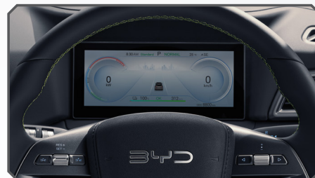
8.8" LCD DIGITAL INSTRUMENT PANEL
